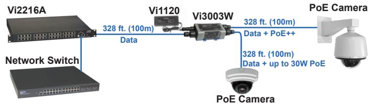
*Vi3003W can provide over 60W PoE on port 2 and 30W PoE on port 3 using Vi1120 external power supply.*
