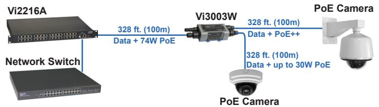
*Vi3003W allows for the transmission of two cameras over a single camera run or adding a new camera close to an existing camera.*
