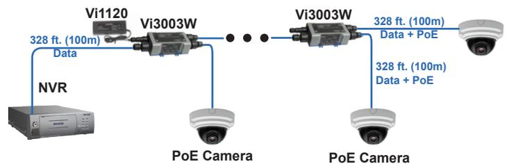
*A total of 9 IP addresses can be accessed on a single cable run, eliminating the need for network switches.*
