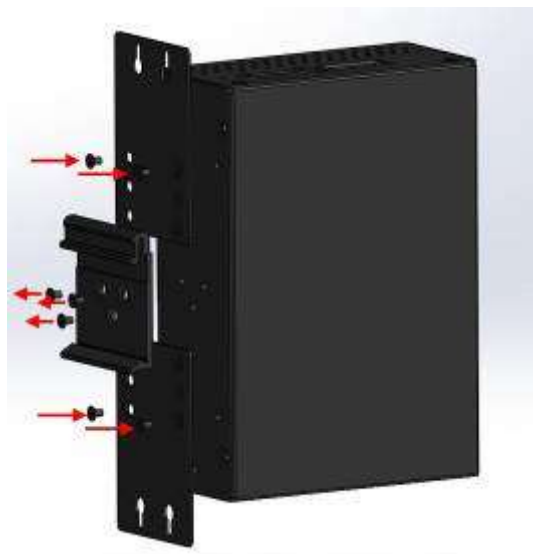
Figure 3.4: Remove DIN-Rail Bracket from the Switch
