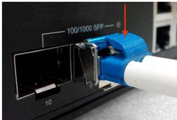
Figure 2.12: Remove LC Connector
