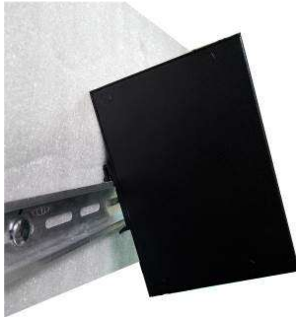
Figure 3.2: Insert the Switch on the DIN-Rail
