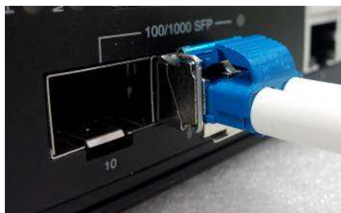
Figure 2.11: LC Connector to the Transceiver
