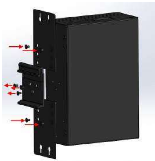
Figure 3.4: Remove DIN-Rail Bracket from the Switch
