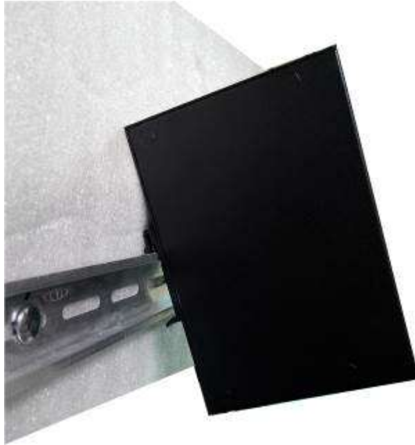
Figure 3.2: Insert the Switch on the DIN-Rail
