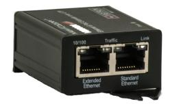
The devices of the VI-UTP-2300A series transmit 10/100Mbps Ethernet and PoE/PoE+ with UTP or Cat cable up to a distance of 500m. The Pass Through technology makes it possible to pass on the PoE power supply, e.g. of a midspan, directly via UTP or Cat cable. The devices do not need any software configuration. Diagnostic LEDs provide an overview of the operating status. The modules of the VI-UTP-2300A series can be mounted as desktop models, on DIN rails and in 19" cabinets.
